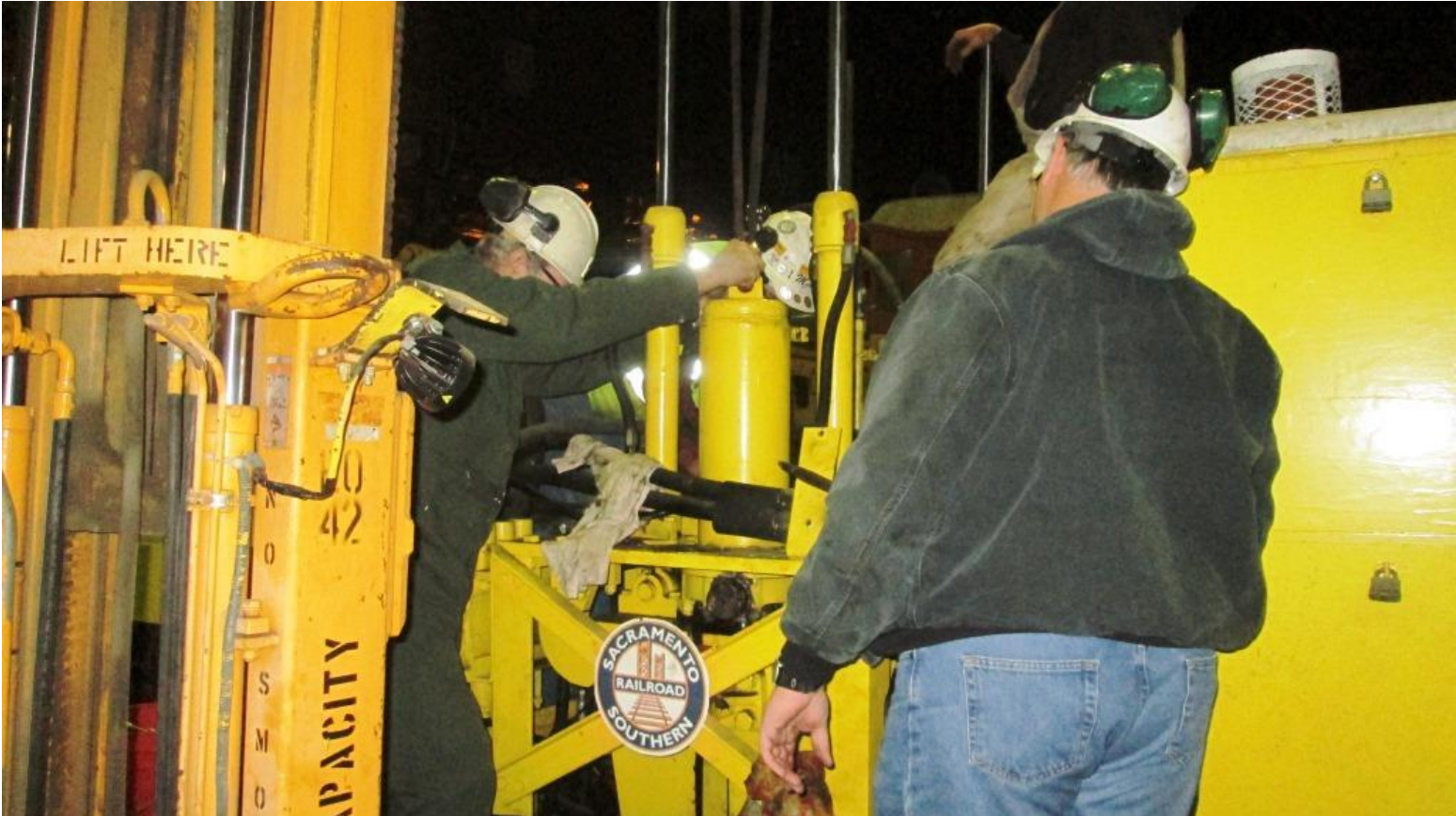
Alan, Mike F., and Chris prepare for the shear lift-cylinder to be removed
